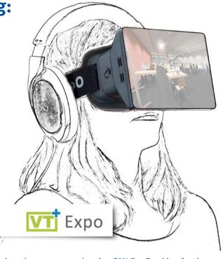
VTplus GmbH has created a virtual exposure solution for anxiety therapy research using SMI Eye Tracking for the Oculus Rift DK2 head-mounted display.
